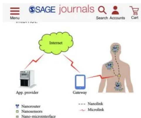
Figure 1 Network architecture for the proposed IoNT application model.
